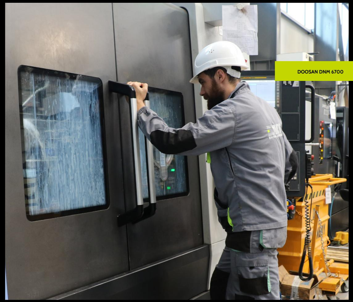
The machine can process parts of complex shapes (foot plates, stars for chain, knives for valves, etc.) with dimensions up to 670 x 1.300 mm.
