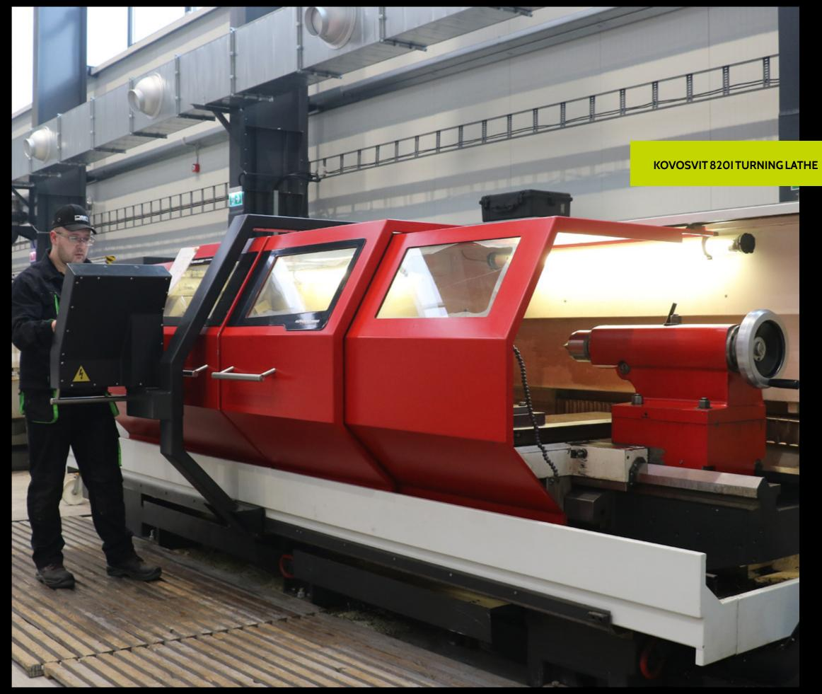
The machine can process parts of complex shapes (like warping head, bronze bush, shafts etc.) with dimensions up to 670x900 mm.
