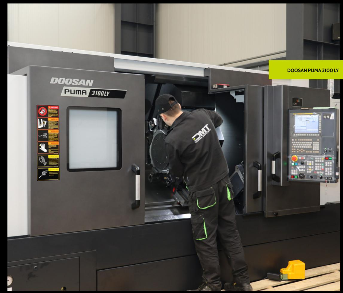
The machine can process parts of complex shapes (like hydraulic cylinders, bronze bush, etc.) with dimensions up to 670 x 900 mm.
