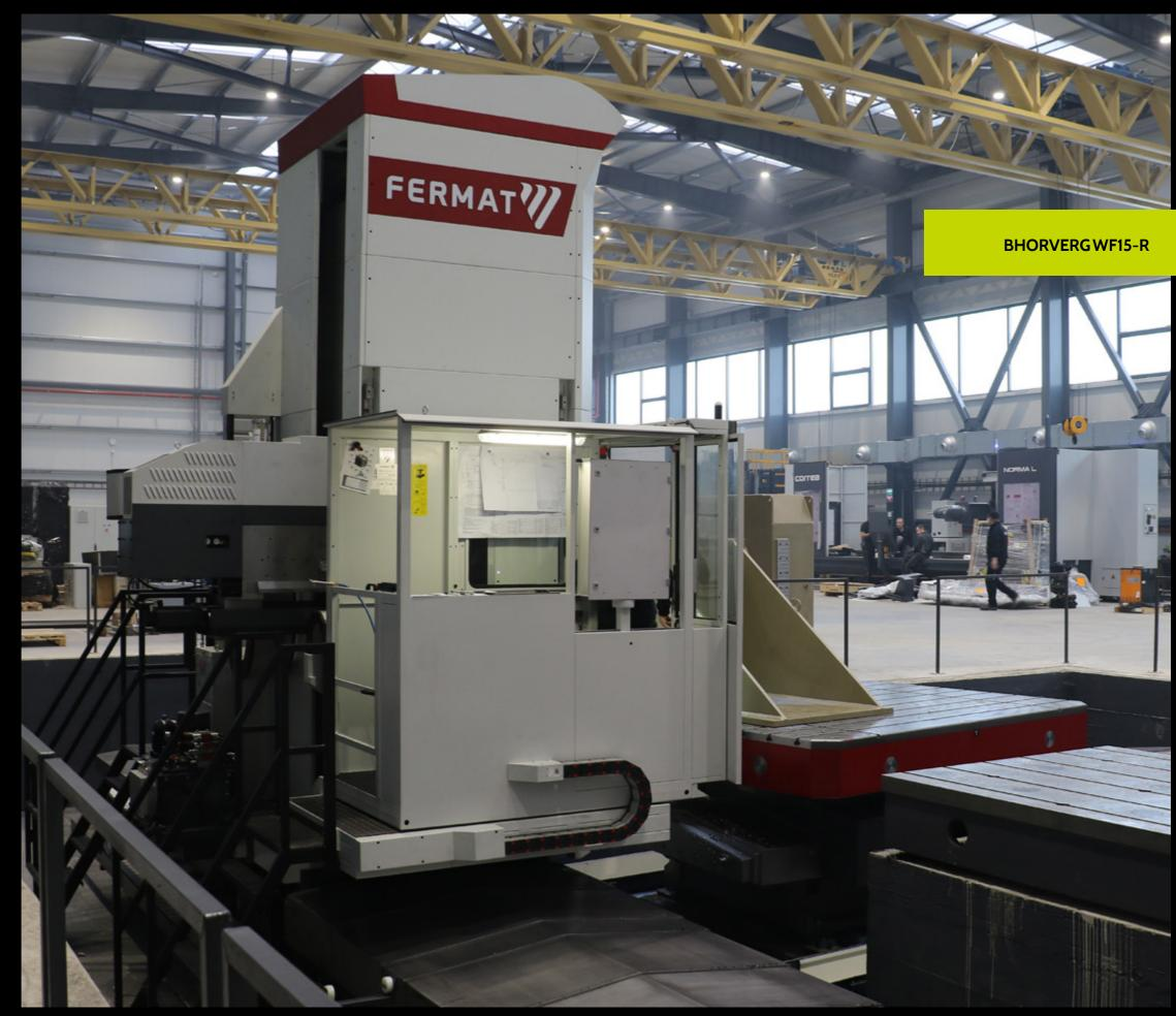
The machine can process parts up to 25 tons, surfaces of maximum 7,700 x 3,000 mm and holes on depths of maximum 730 mm with high accuracy due to numerical control. It is also possible to process inner conical surfaces, threads as well as other complex profiles (ex lateral suport foundation gear cases, etc.).
