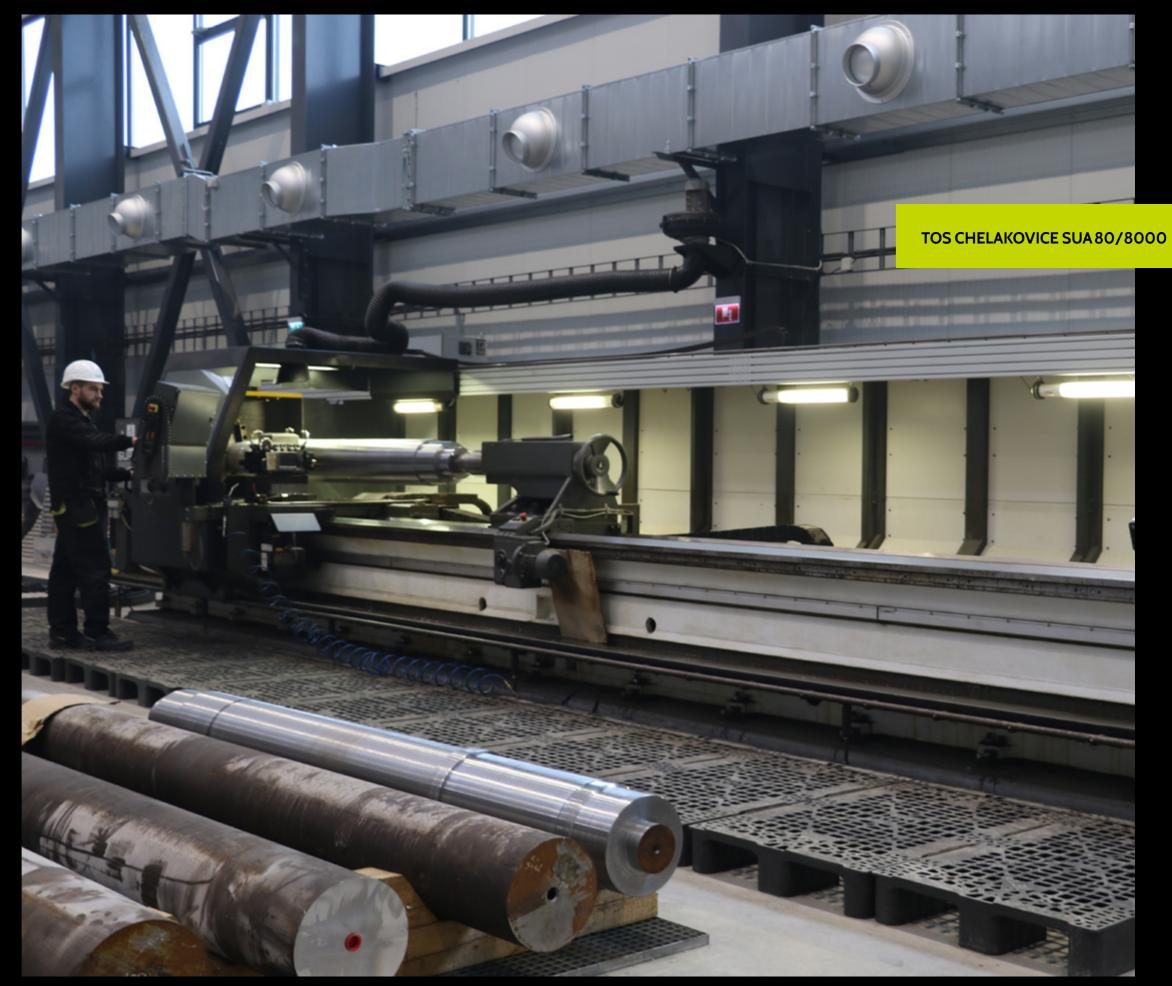
The machine can process parts of complex shapes (like warping head, bronze bush, shafts etc.) with dimensions up to  $520 \times 8.000$  mm.
