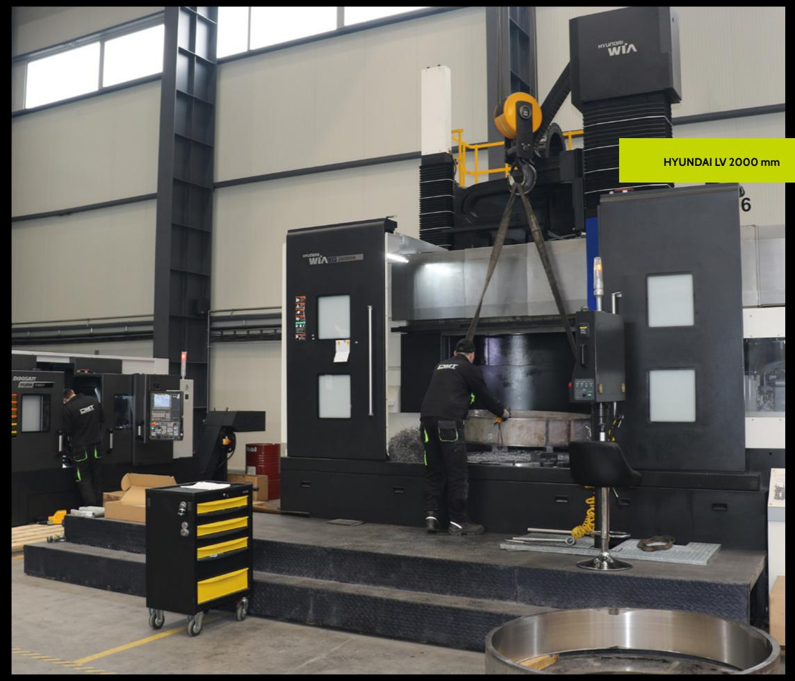
The machine can process parts of complex shapes (like drums, flanges, bronze bush, shafts etc.) with dimensions up to  $2.000 \times 1.600$  mm.
